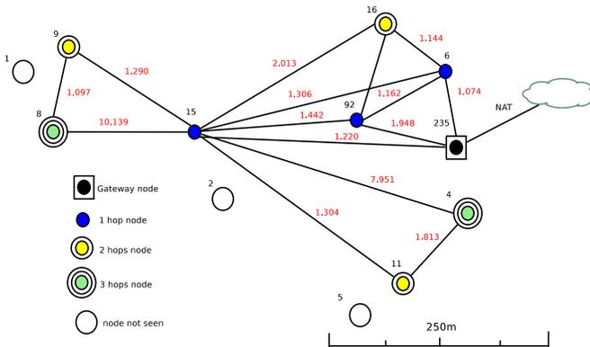
**Figure 5:** Scaled snapshot of the miam mesh during the 2 week measurement period with ETX values indicated per link. Note that the number hops is determined by the route with the lowest sum of ETX values.
