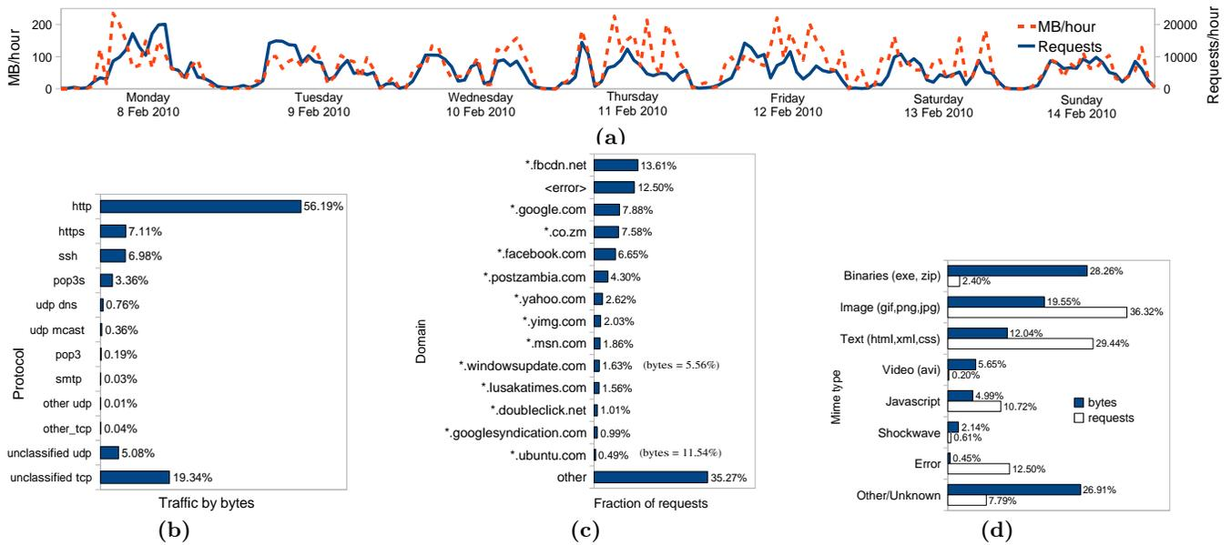
**Figure 2:** Usage analysis over 14 days: (a) Plot of the total web traffic for the satellite link over the second week; (b) Traffic classification by protocol; (c) Web traffic classification by domain visited; (d) Breakdown of traffic by MIME Type.
