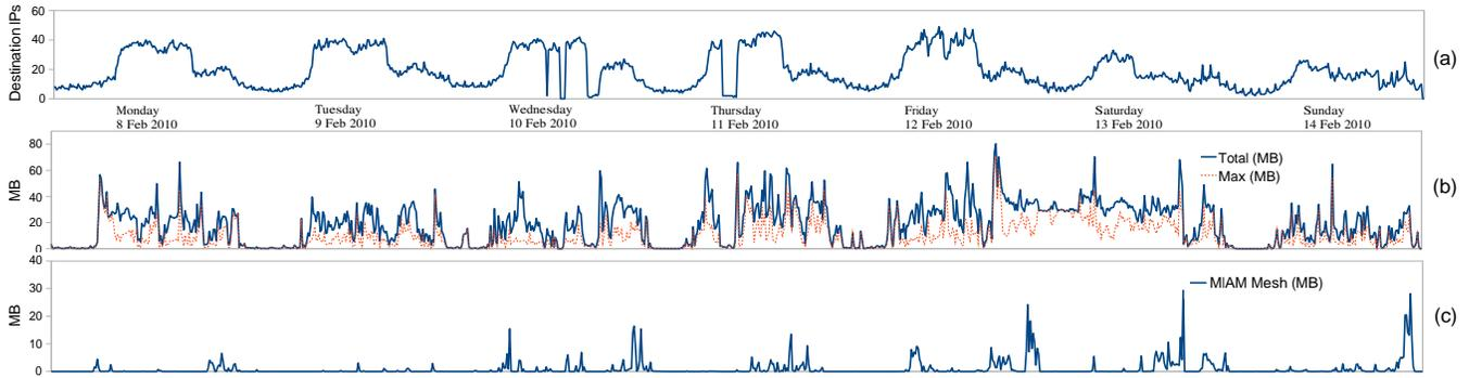
**Figure 4:** The distribution of all inbound traffic on the satellite link in the final week of the 14 day measurement period using 10 minute bins: (a) Total number of unique IP addresses detected; (b) Total traffic vs maximum traffic for a single IP address; (c) Total bandwidth used in the MIAM mesh.
