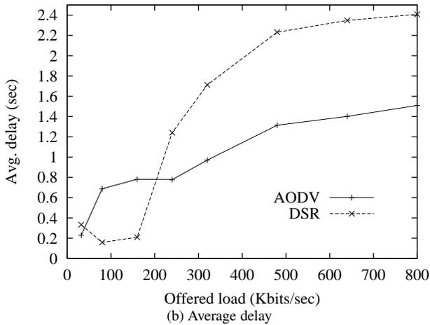
Fig. 8. Performance with increasing offered load with 100 nodes and 40 sources.
