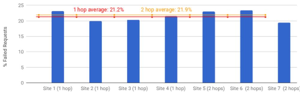
Figure 5: Connection failures by reservation. "Hop" indicates the number of relay towers traveled from the Internet gateway along the backhaul before branching off on unlicensed spectrum. Note averages include connections from devices with indistinguishable user agent strings.
