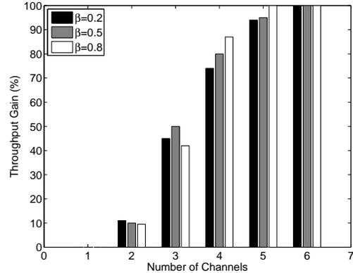
Figure 9. Throughput versus number of orthogonal channels.
