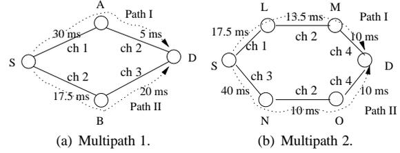
**Figure 2. Two possible sets of multiple paths available from node S to node D.**
