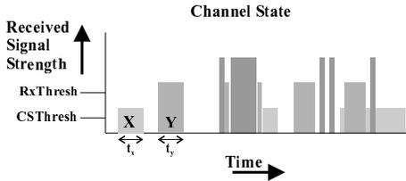
**Figure 4. Diagram of received signal strength versus time.**
