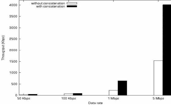
Fig. 7. Throughput comparison with RTS/CTS enabled.
