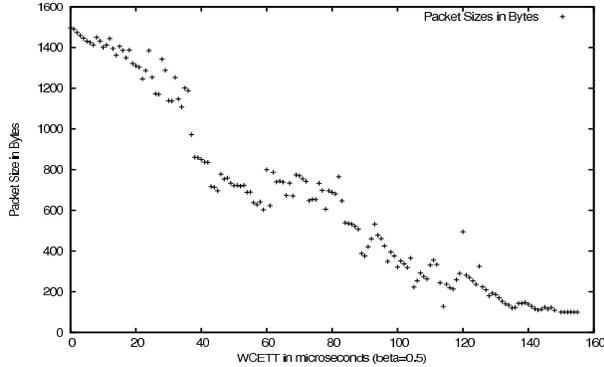
Fig. 3. Mapping of WCETT values to packet sizes.
