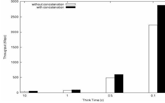
Fig. 8. Throughput measurements with HTTP traffic.
