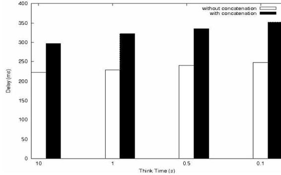
Fig. 9. RTT measurements with HTTP traffic.
