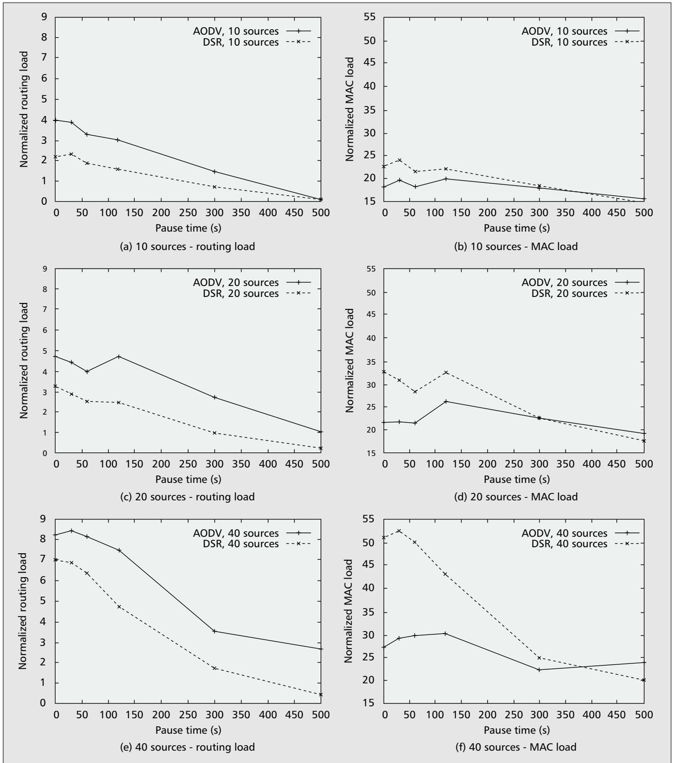
■ **Figure 6.** Normalized routing and MAC loads for the 100-node model with various numbers of sources.
